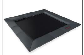
The tiles are molded in grey SBR recycled rubber, Styrene Butadiene Monomer rubber, and the KOMPAN logo is made of EPDM Ethylene Propylene Diene Monomer. Inside each of the rubber tiles there is a 3 mm hot dip galvanized steel plate.
